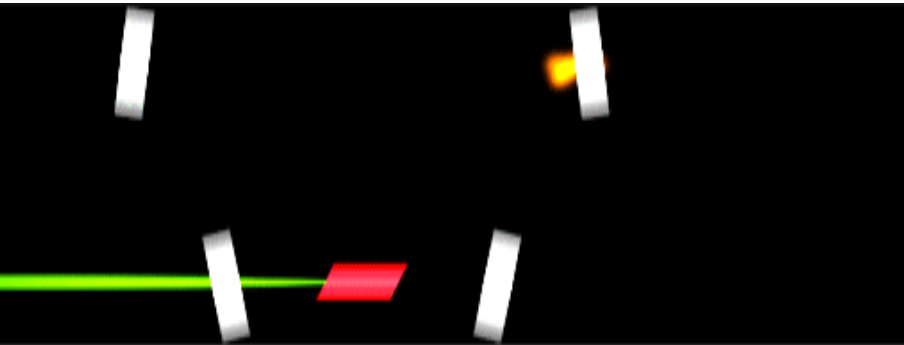
Femtosecond Ti:Sapphire laser, the heart of the femtosecond laser frequency comb
