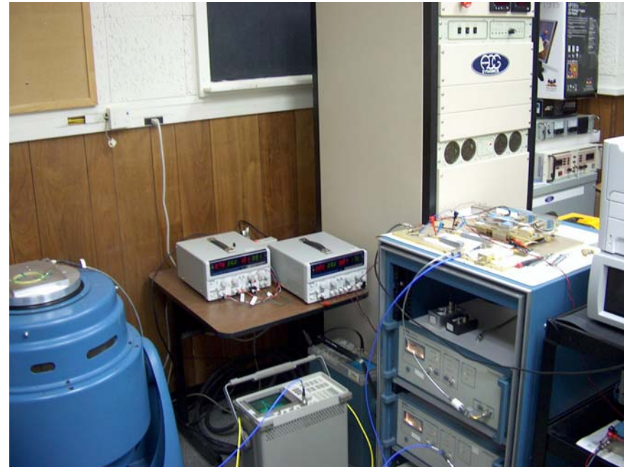
Noise measurement with vibration controller and amplifier, actuator, adaptor, power converter.
